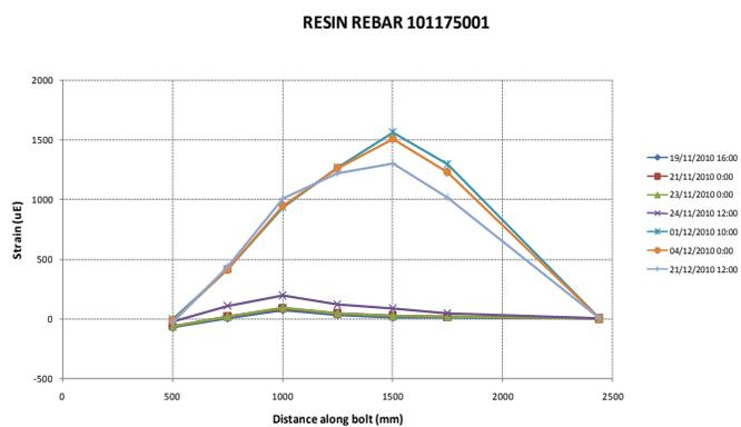
**Figure 18: Strain along the length of rebar**
