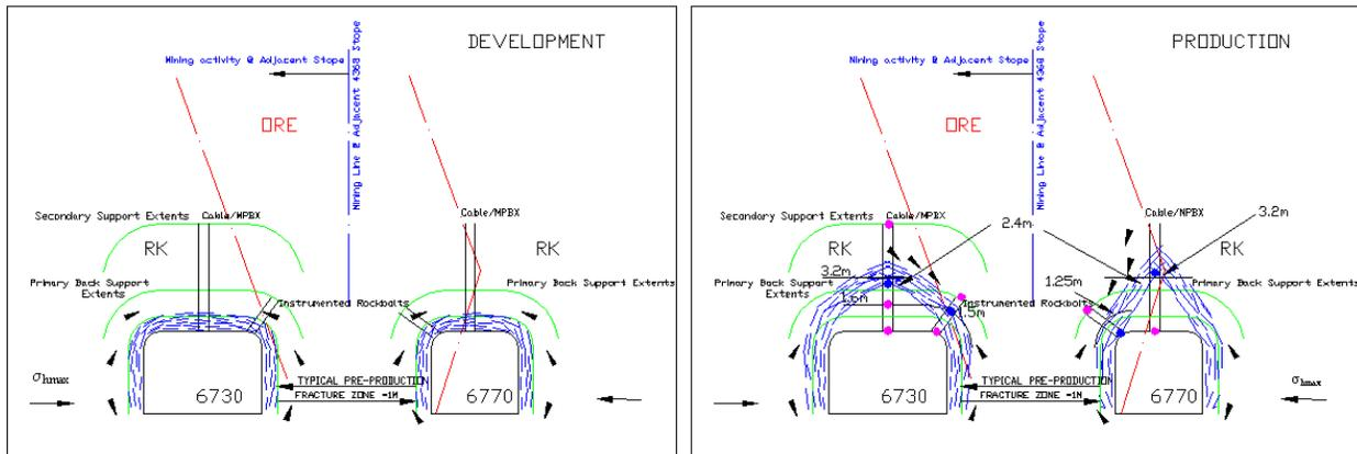
**Figure 21: Induced fracture pattern around a development heading Creighton Deep**
