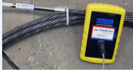
The RS485 output signal can be transmitted over 500m without amplification. Readings (one for each strain gauge) are directly in tons allowing immediate interpretation of cable load without having to enter the raw voltage data in a spreadsheet.
