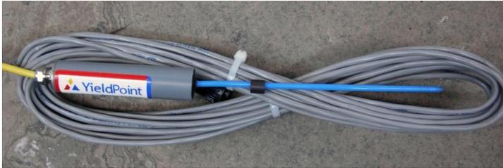
YieldPoint's **d-GMM (SPECTRE)** displacement sensor integrates magnetostrictive technology to produce a high precision digital instrument comprising a non-contact displacement sensor and digital temperature sensor. An on-board microcontroller applies temperature compensation and outputs a digital signal. Both the resolution (<0.01mm) and accuracy (0.25% linearity typical) are significantly better than for similarly priced technology.
