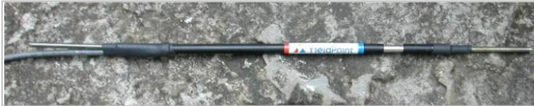
YieldPoint's *d-micro* technology is a high precision digital strain-gauge that can monitor either discrete displacements (*i.e.* crack dilation) or distributed strains (*i.e.* stretch of a steel reinforcing element) to  $\mu\text{m}$  resolution.
