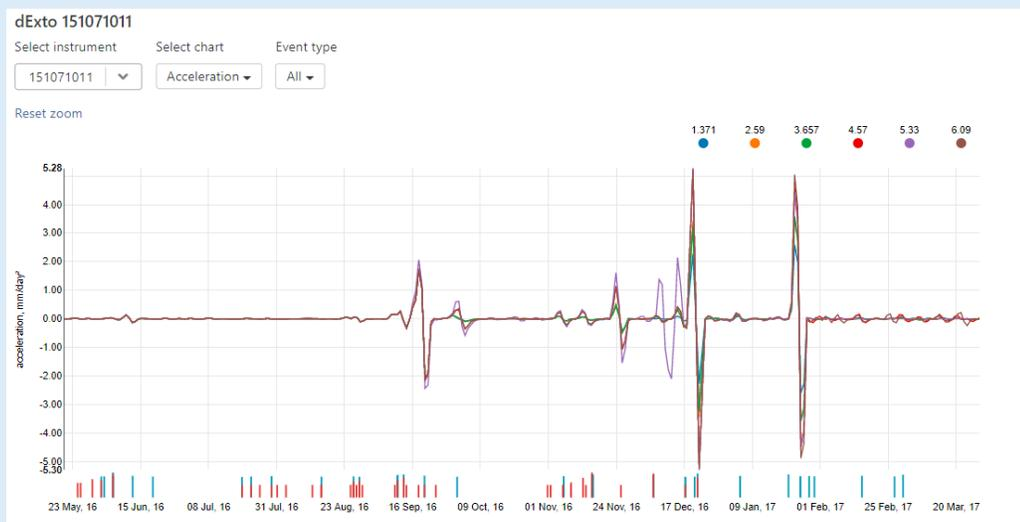
Time series analytics can potentially be used to create forward looking predictions based on future planned blasting events. YieldPoint will work with customers to provide the GDP on a cloud platform or locally on a mine-site server
