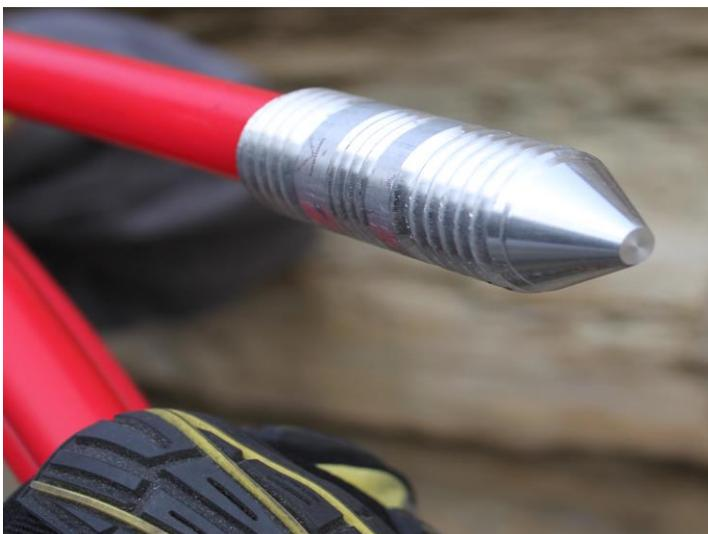
The distal anchor point is tapered to facilitate insertion into the borehole.
